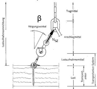
Transport anchor under inclined tensile load-coupling head of the load bearing equipment precision-fitted in a cutout
