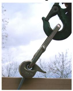
Transport anchor system with the ASSY 4 Combi self-tapping screw and DEHA universal coupling, load group 1-1.3
