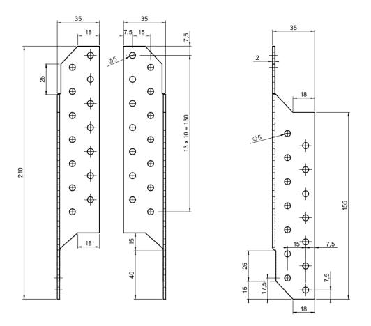
Figure A. 2 Dimensions of Purlin ties 210 right/left
