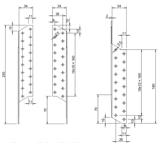
Figure A. 3 Dimensions of Purlin ties 250 right/left
