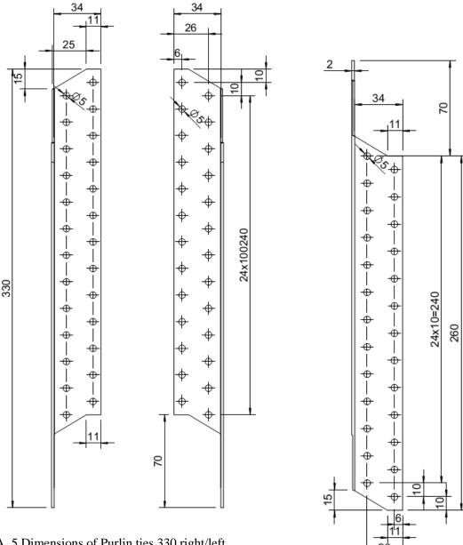
Figure A. 5 Dimensions of Purlin ties 330 right/left
