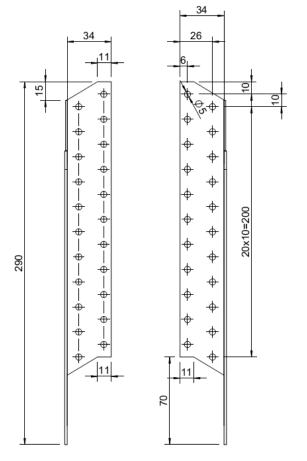
Figure A. 4 Dimensions of Purlin ties 290 right/left
