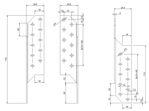
Figure A. 1 Dimensions of Purlin ties 170 right/left
